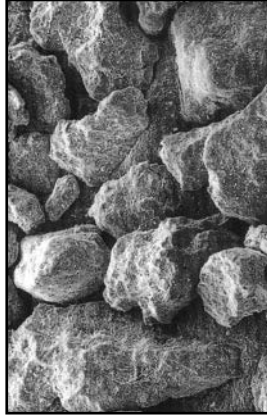
Dry Bentonite, note voids around particles
